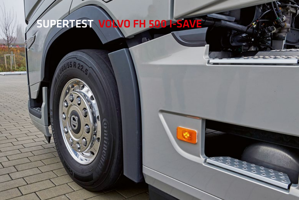
Door interior cladding extended downwards and larger wheel arch covers
