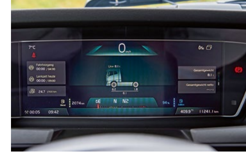
The digital central cluster offers a wide range of options, including an axle load weighing function
