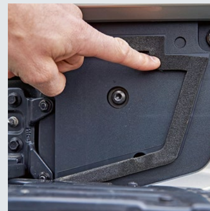
When folded in, the treads of the front step now come up against a soft-foam rubber pad, giving them a better fit
