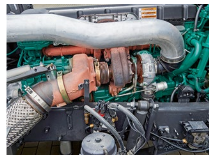
Turbo-compound turbine on engine's right side
