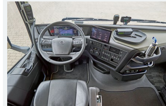
Just right: Volvo's cockpit combines digital features with conventional switches
